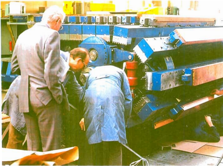
Workers install one of the roller sets for a strip casting line. The copper alloy plates which contact and cool the molten metal are clearly visible in the photograph.
